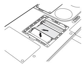
Installing a module
